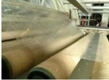
The thin film is stretched out using machines that contain large rollers. These help make the plastic thin and suitable for sweet wrappers.
