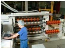
Sometimes the plastic film is coloured and cut into smaller strips on machines like this one. The plastic is crinkly, to wrap around the sweets, and brightly coloured to look attractive.
