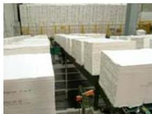
Before it is sent to the plastic factory, it is dried and made into square sheets like blotting paper. This makes it a lot easier to transport to the plastics factory.
